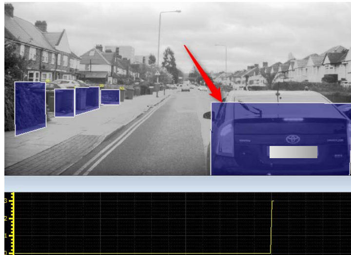
Figure 11 – Example 2 (Subcritical AEB Sequence no. 67): Car immediately brakes after cutting in
