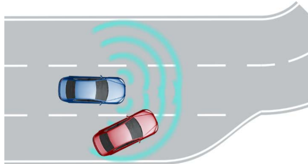
Figure 44 – Front corner radars provide improved view of vehicle cutting in, in front of ego vehicle
