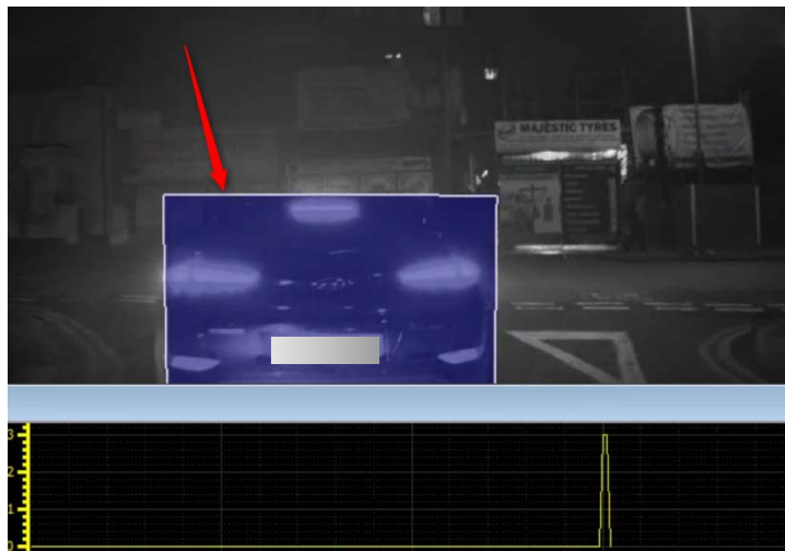
Figure 10 – Example 1 (Subcritical AEB Sequence no. 56): Braking car in front due to approaching a junction
