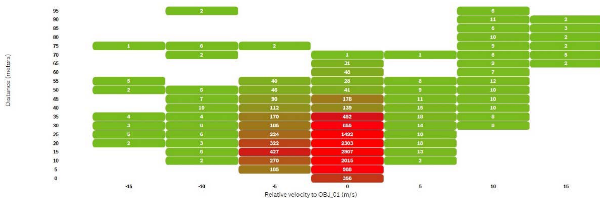
Figure 35 – Heat map - relative velocity of OBJ_01 vs distance
