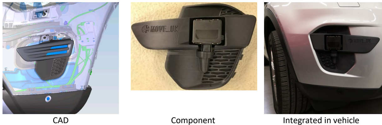
Figure 3 - 3D printed front sensor brackets
